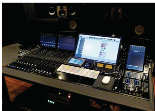
The studio has been equipped with an Avid S6 control surface; TAC Systems VMC-102 controller
