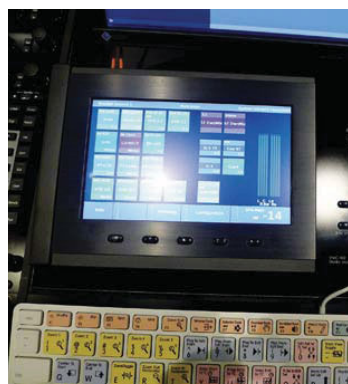
The studio has been equipped with an Avid S6 control surface; TAC Systems VMC-102 controller
